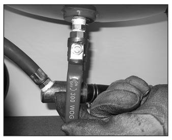
**Figure 14.** Sand metering valve in the full-open position.
